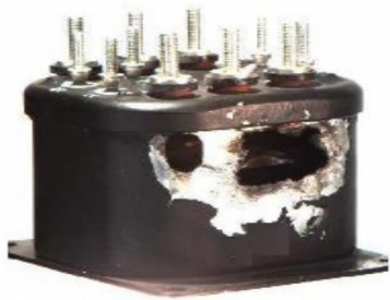
Electromagnetic Relay Vapor Arc Damage
